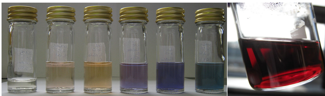
Figure 2: Silver (left) and gold (right) nanoparticle colloids. Differences in particle size cause the silver nanoparticles to display different surface plasmon resonances and hence different colours
